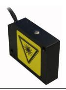
The Laser ride height sensor gives a 0.2 to 4.8V output which is proportional to its displacement above the ground. The displacement is calculated by triangulation from the position of the reflected beam.
